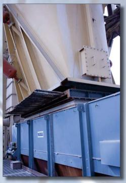
MERRICK's unique multi-parallelogram weigh suspension provides a stable platform for accurate load sensing. The dual load cell weigh suspension spans three pan sections to provide feed rate accuracies of up to +/- 0.5%. Load cells are mounted outboard, allowing for easy access from the sides of the feeder.
